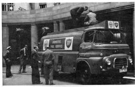
TO MEET the increasing demand for domestic oil fuel from 'private house' customers, a number of specially designed vehicles are being built for service with Authorised Distributors. The vehicles will be equipped with 120 feet of reeled hose and ticket printing meters. The picture shows a vehicle of this type built by Kennings Ltd
